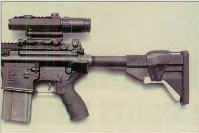
The new AR-10 ARM-TEC pivoting butt stock helped keep the muzzle on target. (below) Mr. Richard Swan, of A.R.M.S., checks out the AR-10 Carbine with his S.I.R. System high in the Rocky Mountains.
